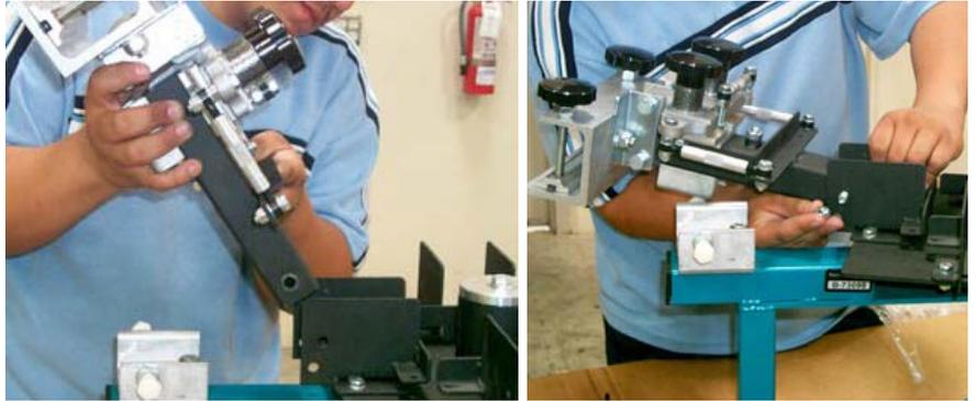
Tighten the top bolt using two 1/2" wrenches.
