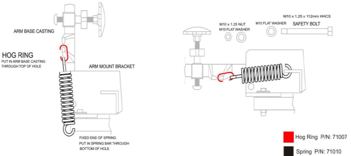
1. Insert hog-ring through the top inside hole in the arm base casting
