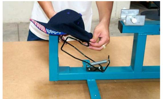
Workhorse Products recommends pulling the sweat band out of the cap to avoid creating an uneven surface on the cap platen.
