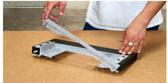
Bend the screen slightly until it fits the contour of the two slots on either side of the ink well.
