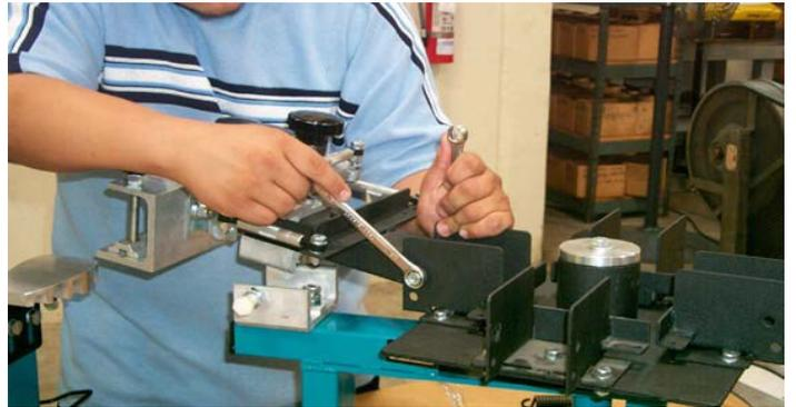
Attach the print head springs by inserting a hog ring with the open end facing the print head into the holes on the spring bracket (on each side of the print head).
