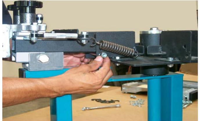
Put a washer on top of the jam nuts and align the four leg leveling bolts (photo 1).
